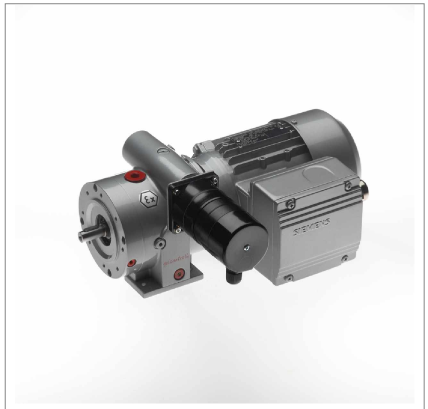
Variable-speed gearbox with ATEX motor "increased safety" for Zones 1 and 21 and electrical remote control for speed adjustment
